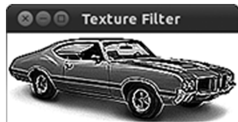
Figure 16.7 The OpenCL kernel sharpens the image by computing a series of two-dimensional dot products.
