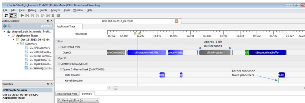
CodeXL snapshot showing the duration of clBuildProgram for a binary kernel
