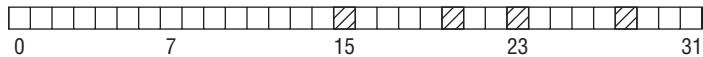
Figure 3-25: Memory fragmentation where few reserved pages prevent the allocation of larger contiguous blocks.
