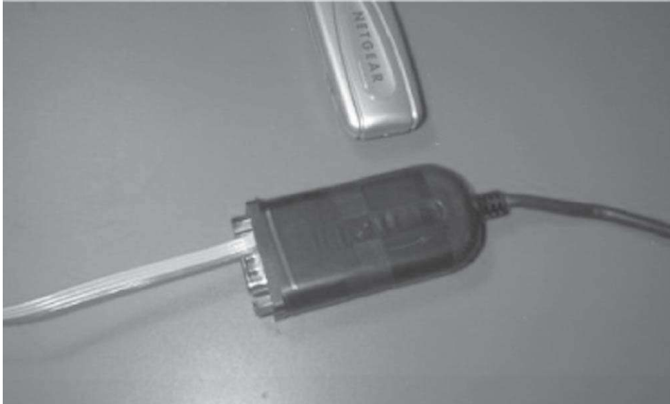
Figure 3.11 Reassembled serial adaptor.
