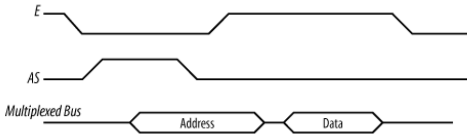
Figure 16-3. Timing of the multiplexed bus on a 68HC11
