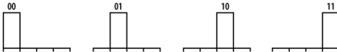
Figure 10-4. 4PPM cell encoding
