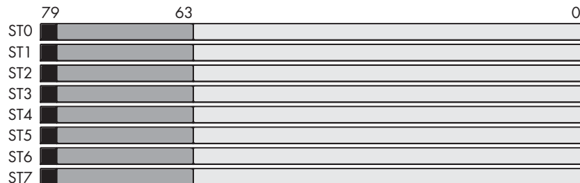
Figure 6-1: FPU floating-point register stack
