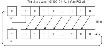
RCL shifts all bits left and moves bit 7 to the Carry flag. The 0-bit previously in the Carry flag is moved into bit 0.
