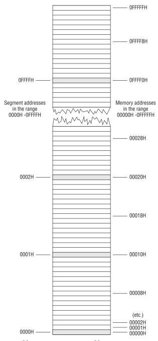
Figure 4-4: Memory addresses versus segment addresses
