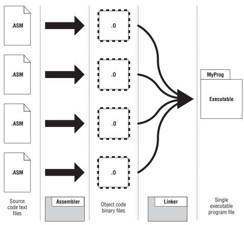
Figure 5-8: The assembler and linker
