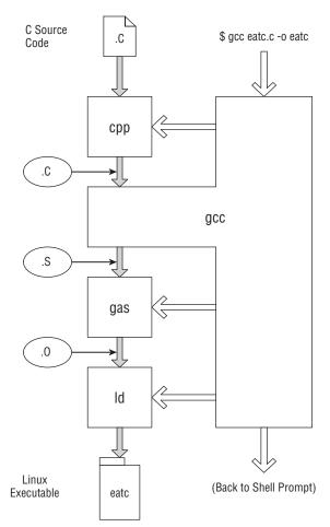
Figure 12-1: How gcc builds Linux executables
