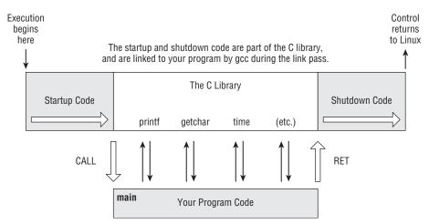
Figure 12-2: Structure of a hybrid C-assembly program
