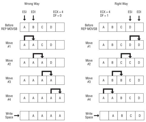
Figure 11-2: Using MOVSB on overlapping memory blocks
