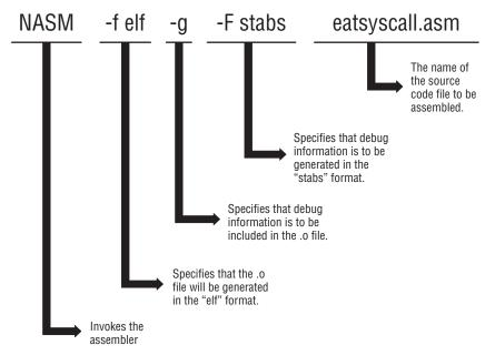
Figure 5-11: The anatomy of a NASM command line
