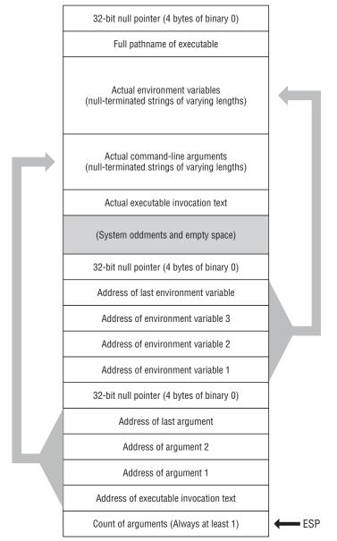
Figure 11-4: Linux stack at program startup
