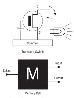
Figure 3-1: Transistor switches and memory cells
