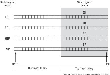
The shaded portion of the registers is what exists on the older 16-bit x86 CPUs: The 8086, 8088, and 80286.
