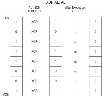
Figure 9-3: Using XOR to zero a register
