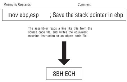
Figure 5-7: What the assembler does
