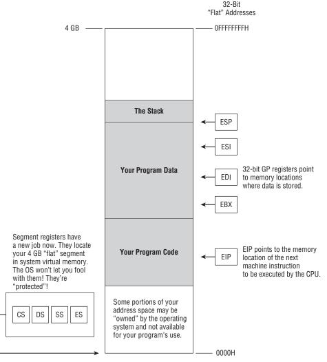
Figure 4-10: Protected mode flat model
