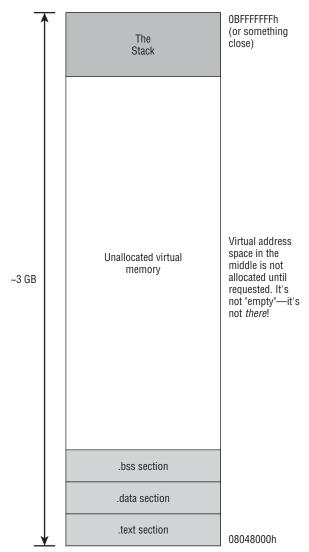
Figure 11-3: A program's virtual memory block at runtime
