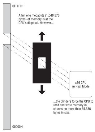
Figure 4-3: Seeing a megabyte through 64K blinders
