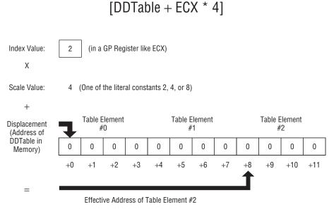
Figure 9-10: How address scaling works
