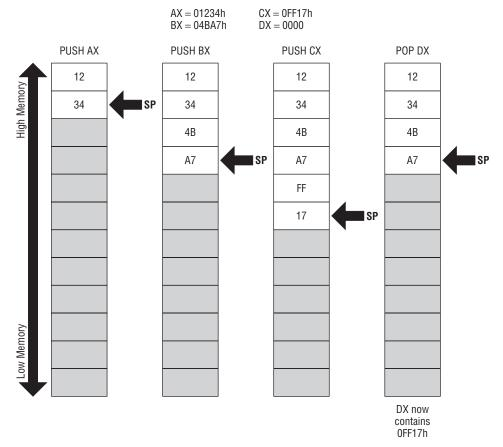
Figure 8-3: How the stack works
