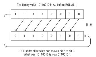
Figure 9-4: How the rotate instructions work
