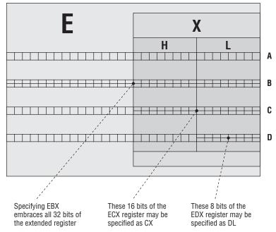
Figure 4-7: 8-bit, 16-bit, and 32-bit registers
