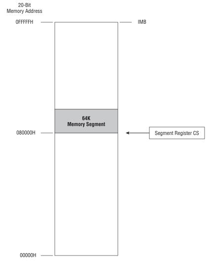
Figure 4-2: The 8080 memory model inside an 8086 memory system
