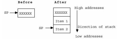
Before the items are pushed, SP points to (holds the address of) the previous item that was pushed. After two new words have been pushed, the stack pointer points to the second of these, and the first word pushed lies 'underneath' it.
