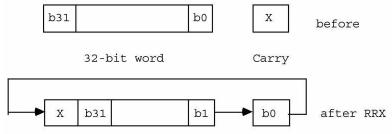
The old bit 0 is shifted into the carry. The old content of the carry is shifted into bit 31.
