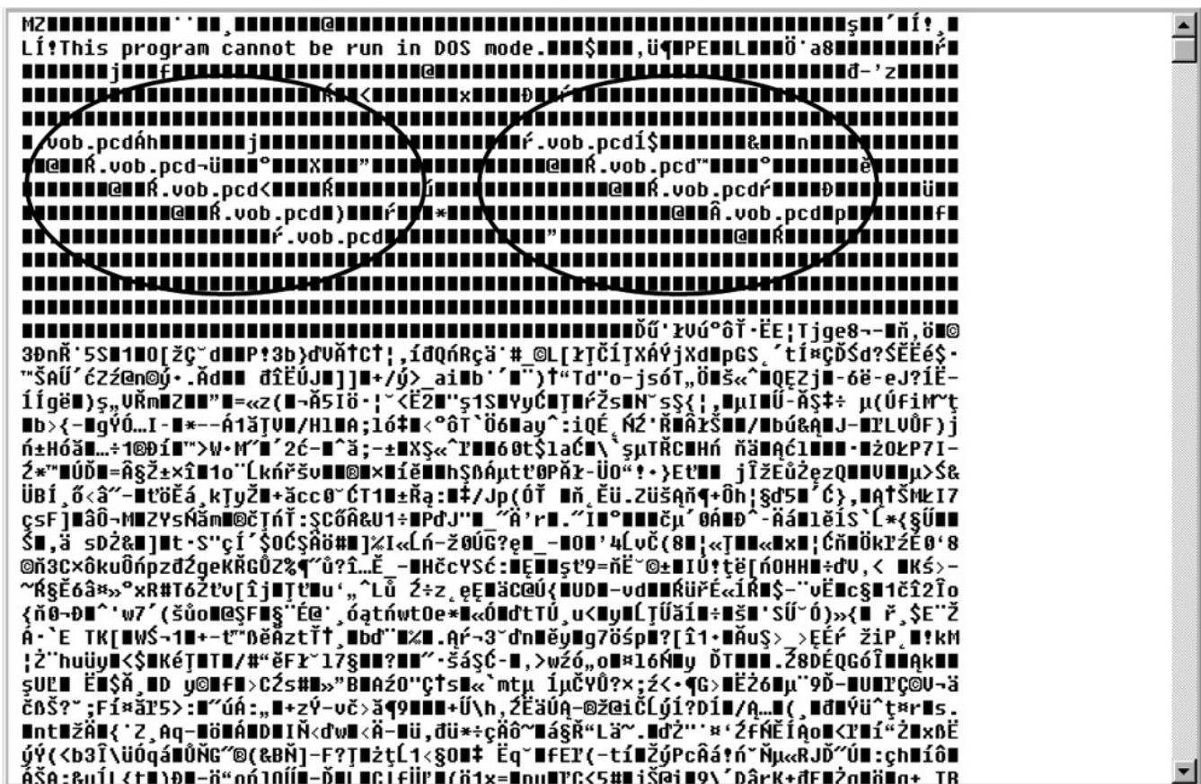
Figure 4.2: VOB is given away by the section name in the PE file header As is common with this type of protection, the program checks for errors on the original CD, which differ on copies. Decoding values for a given product are calculated according to a certain algorithm, and these values are then used to decode the original PE file. Since this is really nothing new, crackers who have managed to remove SafeDisc find it easy to remove VOB as well (see Figure 4.3).
