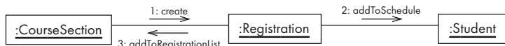
Figure 8.8 A communication diagram representing the same interaction as the sequence diagram of Figure 8.1
