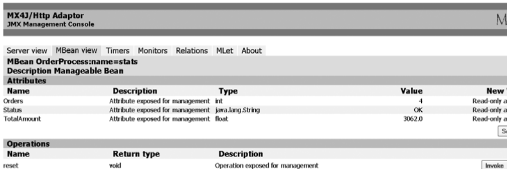
Figure 9-6. Invoking the reset method through the HTTP adapter of MX4J
