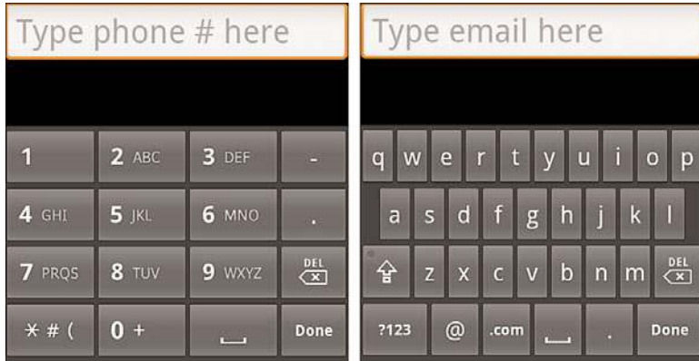
Figure 4.9 Examples of utilizing different soft keyboards when inputText is set as “phone” or “textEmailAddress”.
