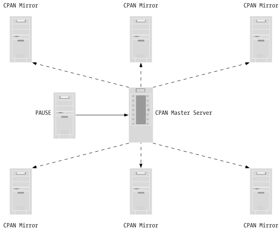
Figure 1-2. The CPAN Network Topology
