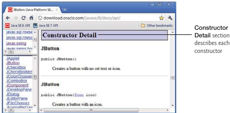
Fig. E.10 | Constructor Detail section of class JButton . (Courtesy of Oracle Corporation)
