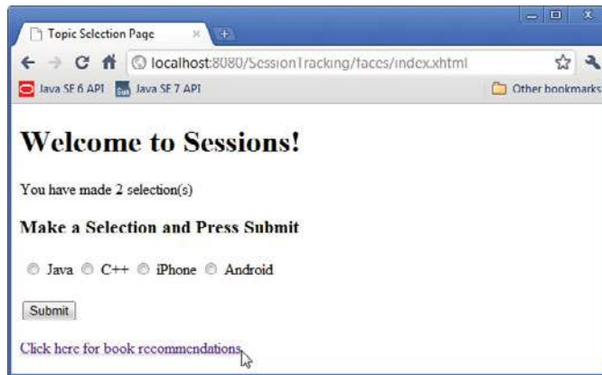
Fig. 29.19 | index.xhtml after the user has submitted the form the second time and is about to click the link to the recommendations.xhtml page.
