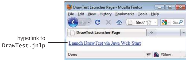
Fig. 23.13 | HTML document that launches the DrawTest applet when the user clicks the link.
