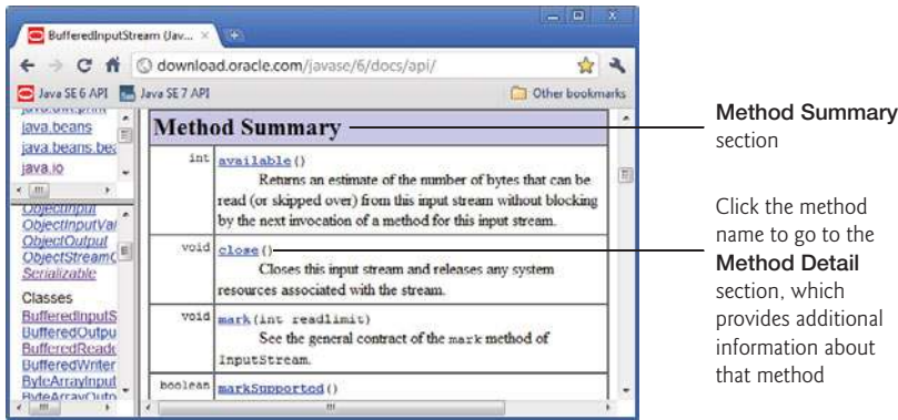
Fig. E.8 | Method Summary section of class BufferedInputStream . (Courtesy of Oracle Corporation)
