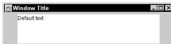
Figure 12-10 The text area GUI element is used to display a block of text or to receive a block of text from the user of your program.
