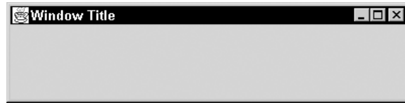
Figure 12-3 You create a window by defining your own window class that extends the JFrame class.
