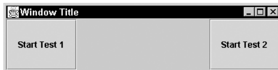
Figure 12-4 The Border Layout Manager divides the container into five areas, known as north, south, east, west, and center.
