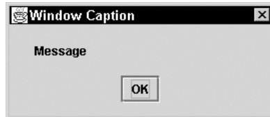
Figure 12-1 Here is a “plain” message dialog box. It is useful for displaying any kind of message on the screen.
