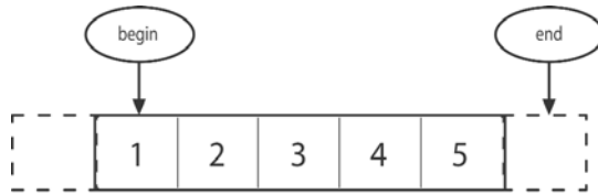
FIGURE 2.5 Beginning and end iterators of a range.
