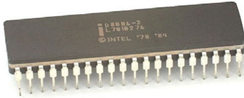
FIGURE 29.1 The Intel 8086 microprocessor.
