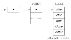
The type description **class** at the right is initialized at compile time. The object is created at run time and the dashed pointers are then inserted. In the assignment
