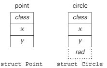
The picture shows that every circle begins with a point. If we derive **struct Circle** by adding to the end of **struct Point**, we can pass a circle to **move()** because the initial part of its representation looks just like the point which **move()** expects to receive and which is the only thing that **move()** can change. Here is a sound way to make sure the initial part of a circle always looks like a point:
