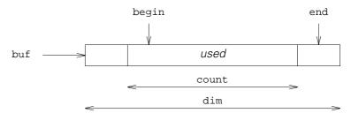
**begin** and **end** limit the used part of the list, **dim** is the maximal buffer size, and **count** is the number of elements currently stored in the buffer. **count** makes it easy to distinguish between a full and an empty buffer. Here is the class description *List.d*:
