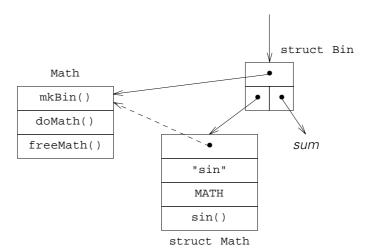
We let the left side of a binary node point to the symbol table element for the function and we attach the argument tree at the right. The binary node has **Math** as a type description, i.e., the methods **doMath()** and **freeMath()** will be called to execute and delete the node, respectively.
