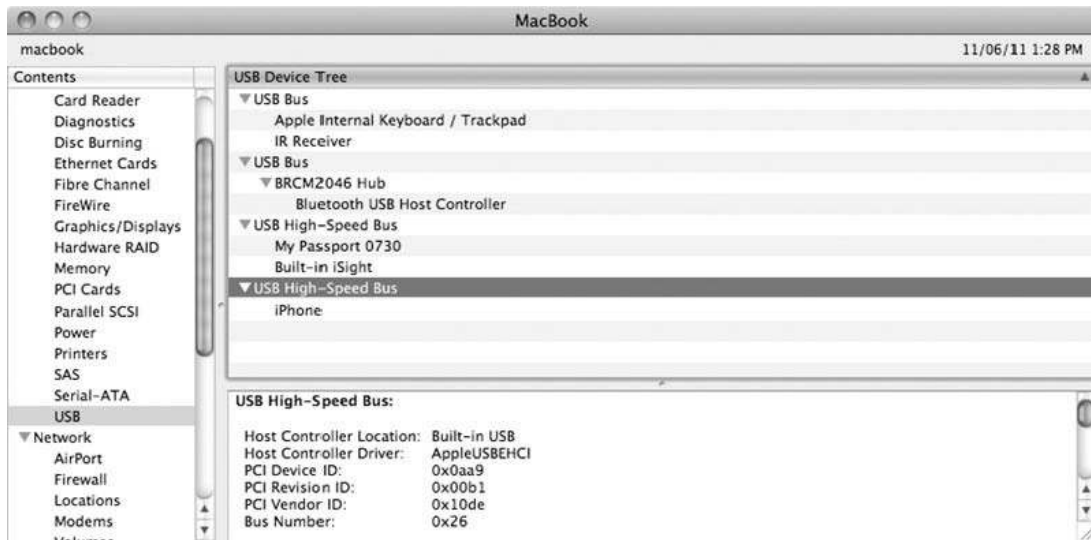
Figure 8-1. System Information showing the USB topology of a MacBook, with external devices connected
