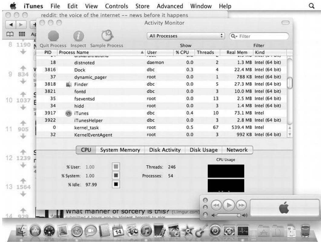
Figure 1-3. Activity Monitor on Mac OS X showing all processes running on the system. Compare this to the Dock, which shows the visible user applications.
