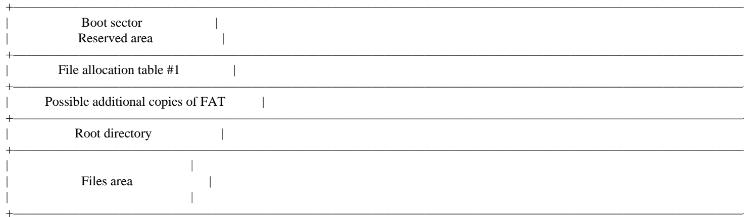
Figure 10-1. Map of a typical MS-DOS logical volume. The boot sector (logical sector 0) contains the OEM identification, BIOS parameter block (BPB), and disk bootstrap. The remaining sectors are divided among an optional reserved area, one or more copies of the file allocation table, the root directory, and the files area.
