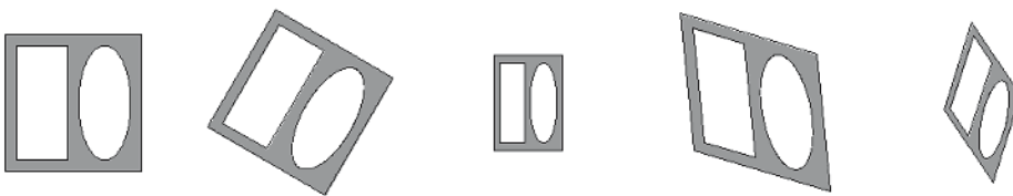
Figure 7-29. From the left: original, rotated, scaled, sheared, and all at once
