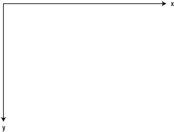
Figure 7-1. The x value increases from left to right; the y value increases from the top downward.
