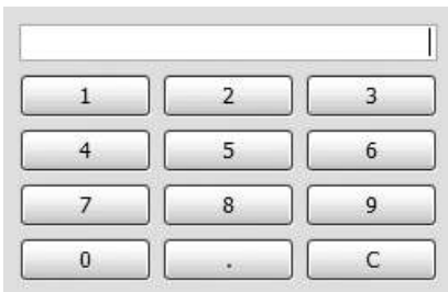
Figure 6-1. A keypad made from a QLineEdit and a set of QPushButton widgets
