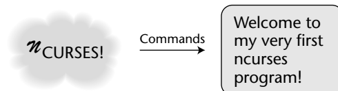
Figure 2-1: The standard screen is the default window for NCurses text output commands.
