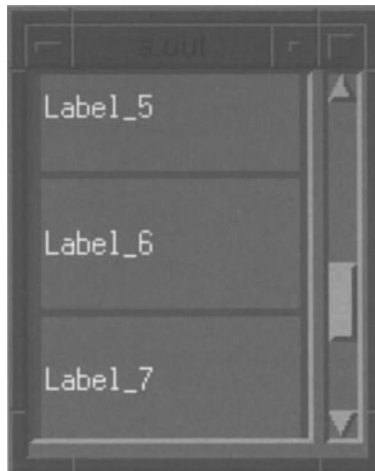
Figure 10.4. Row-column inside scrolled-window
