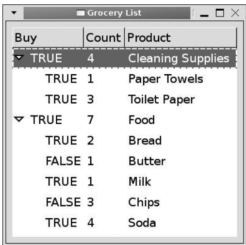
Figure 8-5. A tree view widget using a GtkTreeStore tree model
