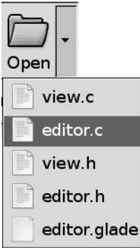
Figure 9-6. A menu tool button showing recently opened files
