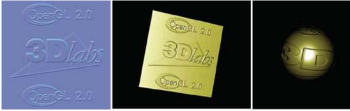
Figure 8.10 Normal mapping (A normal map (left) and the rendered result on a simple box and a sphere. (3Dlabs, Inc.))
