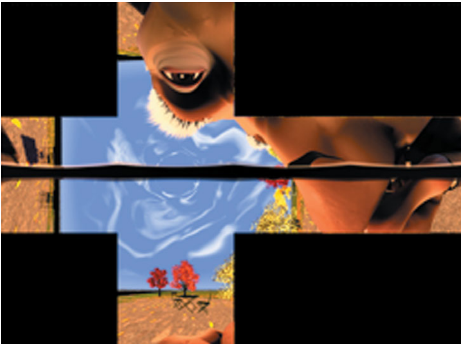
Color Plate 24 Reflection map from environment computed from the center of the lens on Geri's glasses. The reflection map is then mapped to the glasses as part of the rendering process.
