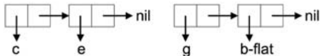
Figure 3.4.2: List cell representation of inputs to cons , list , and append : {c e}, {g b-flat}
