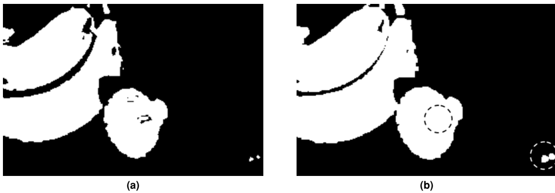
Figure 10.38: Binary image object size variation with dilation. (a) Original binary image with a few objects of Figure 10.36. (b) After three dilation operations.
