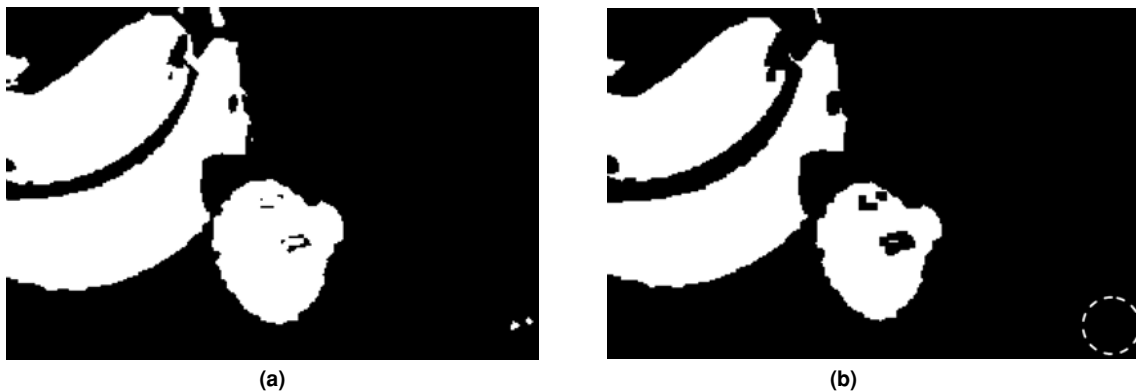
Figure 10.40: Binary image object size variation with erosion. (a) Original binary image of with a few objects of Figure 10.36. (b) After three erosion operations.
