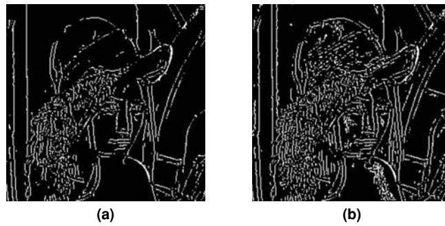
Figure 10.23: Lena image, Canny edge detection with various parameters: (a) T1 = 16 , T2 = 32 , Sig = 1.0 . (b) T1 = 8 , T2 = 16 , Sig = 2.0 .
