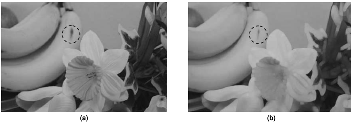
Figure 10.37: Grayscale image intensity variation with dilation. (a) Original image. (b) Intensity variations with three dilation operations.
