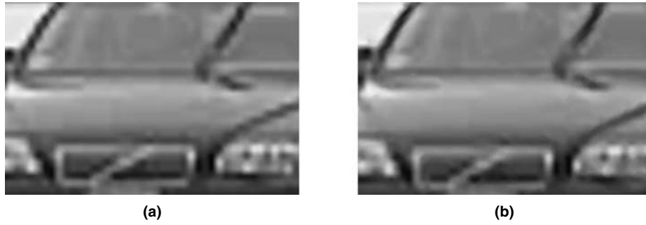
Figure 15.3: Video scaling. (a) Using bilinear interpolator. (b) Using nonlinear interpolator.
