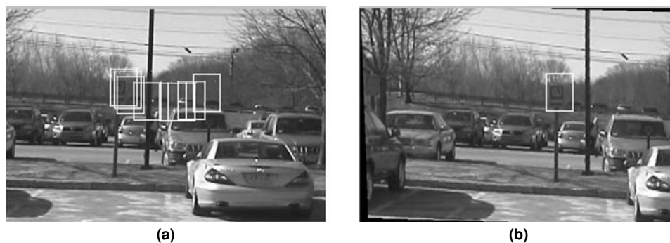
Figure 11.24: Digital image stabilization simulation results. (a) Unstabilized video sequence. (b) Stabilized video sequence.
