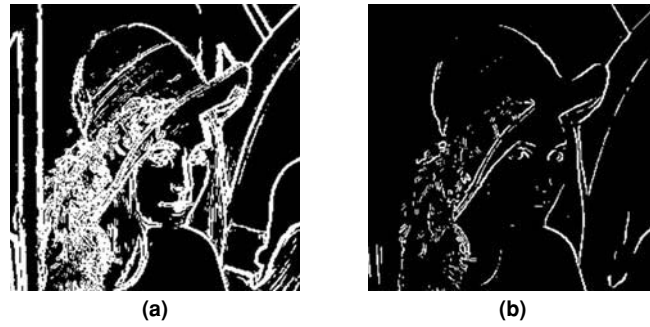
Figure 10.12: Lena image, Sobel edge detection with various thresholds. (a) T = 64 . (b) T = 240 .
