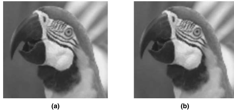
Figure 15.16: Video chroma scaling. (a) Bicubic interpolation. (b) Bilinear interpolation.
