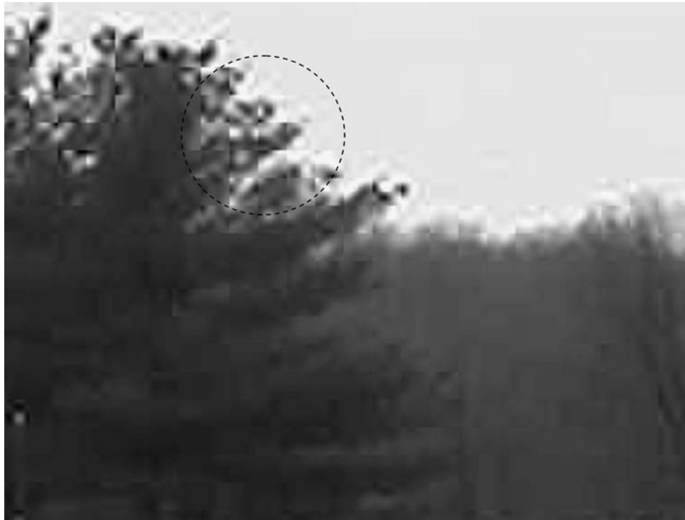
Figure 14.39: Decoded video before filtering with deblock filter.
