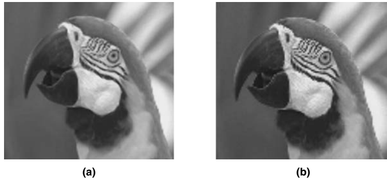
Figure 15.14: Video scaling. (a) Edge-based interpolation. (b) Bilinear interpolation.
