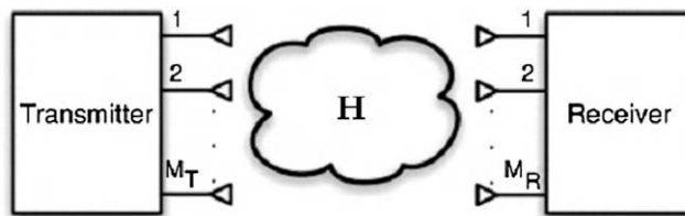
Figure 5-1: Multiple antenna (MIMO) system.
