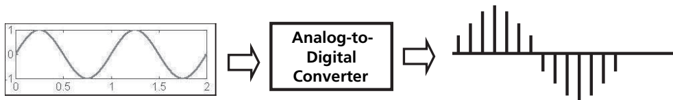
Figure 4.7 Analog-to-digital conversion for signal processing
