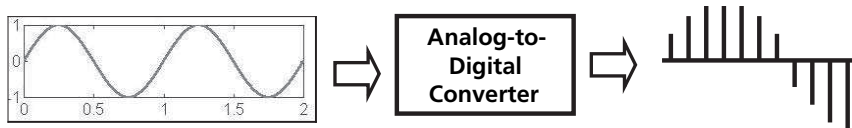
Figure 1.3 Analog-to-digital conversion for signal processing
