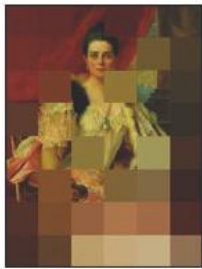
QBIC interprets the virtual canvas as a grid of coloured areas, then matches this grid to other images stored in the database.
