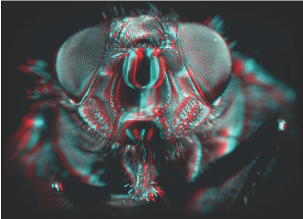
Figure 1.70 Red/cyan stereo image of a fly's head. This image was captured as two separate SEM images, which were then superimposed as different color channels. To view the image, use glasses with a red filter in front of the left eye and a green, cyan, or blue filter in front of the right eye.
