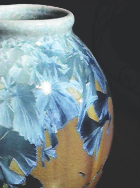
Figure 15.2 Photograph of a glaze covering a ceramic pot. The glaze flows down the surface in a molten state and solidifies to an amorphous glass under the forces of surface tension. Subsequently, the atoms rearrange themselves to form crystals which nucleate and grow in the glaze, producing visually interesting patterns and also altering the surface relief.
