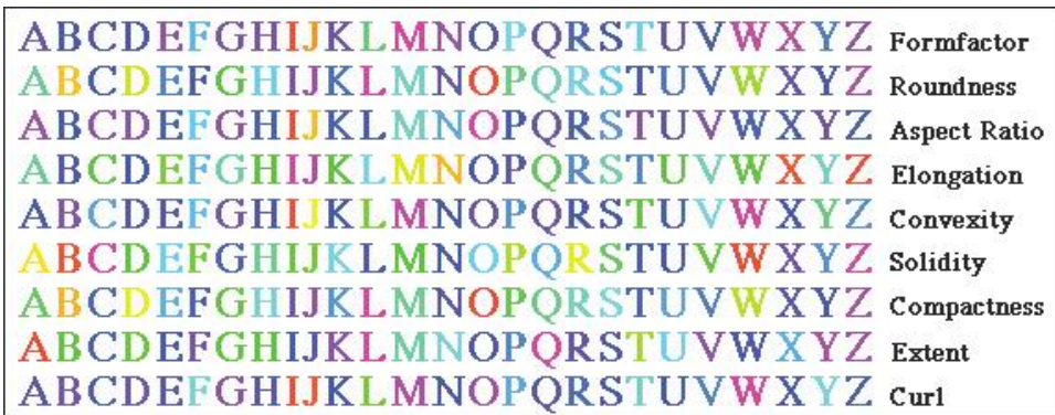
Figure 11.9 Measurement of a series of shapes (letters of the alphabet). In each row, the colors of the features code the relative numeric value (red = high, magenta = low) of a different shape parameter, corresponding to the labels.
