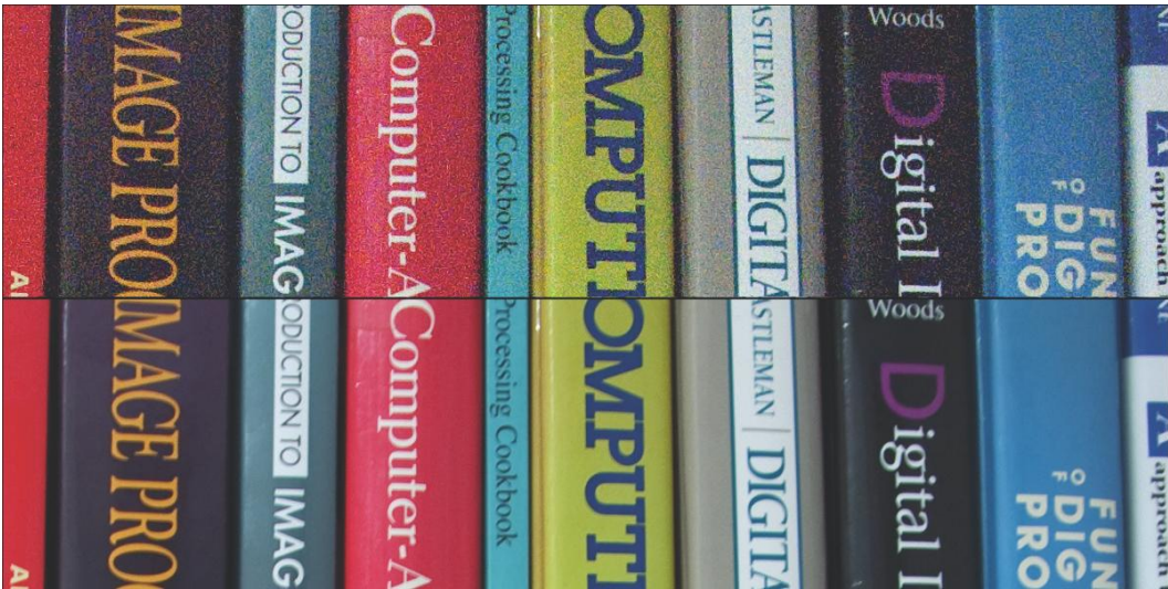
Figure 1.26 The same image recorded with an ASA setting of 1600 (top) and 100 (bottom), showing the increase in random pixel noise produced by higher gain in the camera.
