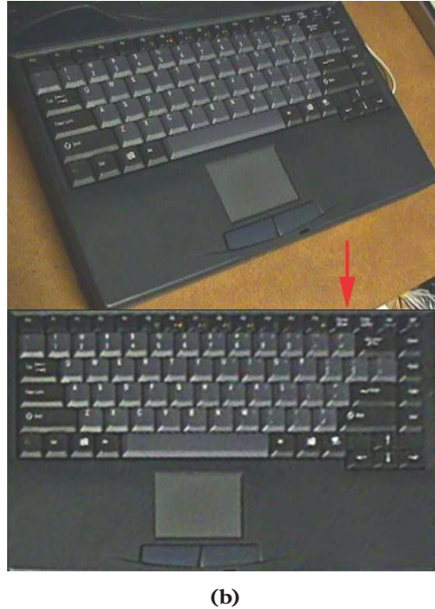
Figure 1.79 Geometric distortion occurs when a surface is viewed from a position away from the surface normal. Correcting this distortion to obtain a rectilinear image which can be properly processed and measured, or fitted together with adjoining images, requires knowing the viewing geometry and/or including known fiducial marks in the scene that can be used to determine it.
