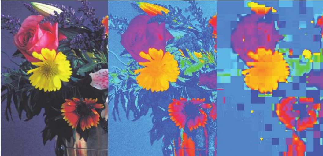
Figure 3.24 Effect of JPEG compression on colors (from left to right): original image; hue channel from the original with saturation set to maximum to show colors varying from pixel to pixel; hue channel after 30:1 JPEG compression, showing that the hue values are uniform over large blocks.
