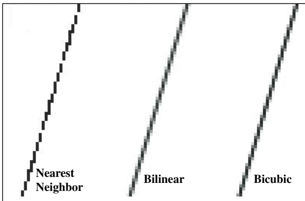
Figure 4.70 Effect of rotating a one pixel wide black line using nearest neighbor, bilinear, and bicubic interpolation.
