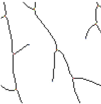
Figure 8.72 Detail of a skeleton showing nodes. Removing the red node points does not disconnect all of the branches; for some pixel configurations, the green “near-node” points must also be deleted to assure that no 8-connections remain between different branches.
