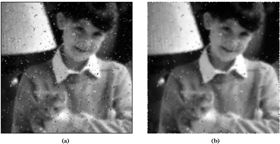
Figure 4.30 Application of Olympic filter to shot noise. The original image is shown in Figure 4.16b : (a) the 2 brightest and 2 darkest pixels in each 3 \times 3 neighborhood are ignored and the remaining 5 averaged; (b) the 4 brightest and 4 darkest pixels in each 5 \times 5 neighborhood are ignored and the remaining 17 averaged.
