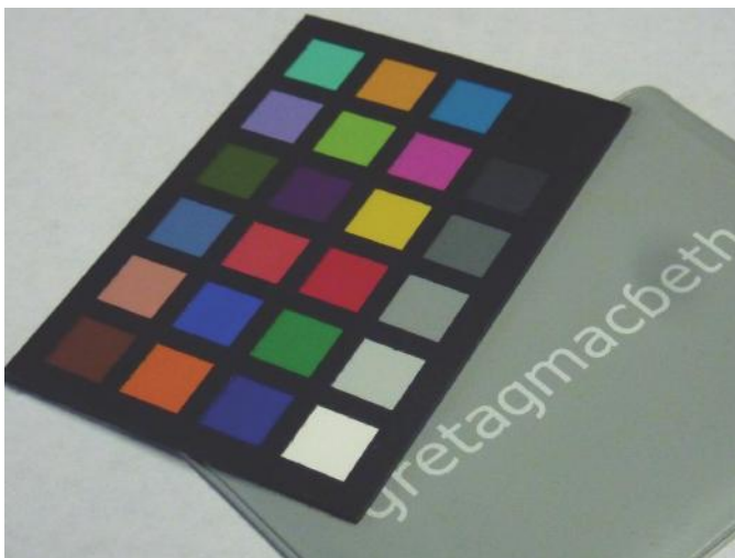
Figure 1.48 The GretagMachbeth ColorChecker® chart. The colors are not reproduced in this text adequately for use as a chart, and this figure is illustrative only. The colors are, in order from the left corner: dark skin, light skin, blue sky, foliage, blue flower, bluish green, orange, purplish blue, moderate red, purple, yellow green, orange yellow, blue, green, red, yellow, magenta, cyan, white, neutral 8, neutral 6.5, neutral 5, neutral 3.5, and black.
