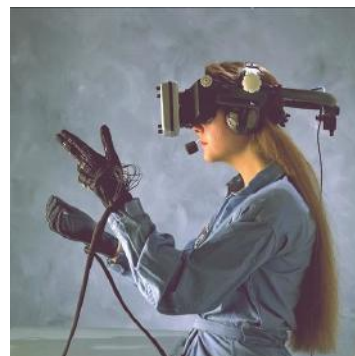
Figure 14.39 An example of immersive virtual reality, involving a head mounted stereo display and datagloves that provide 3D manipulation of objects.
