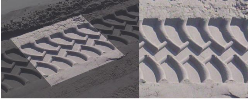
Figure 4.61 Outlining a region parallel to the edges of the tire track defines the image distortion, from which the necessary rectification can be calculated.
