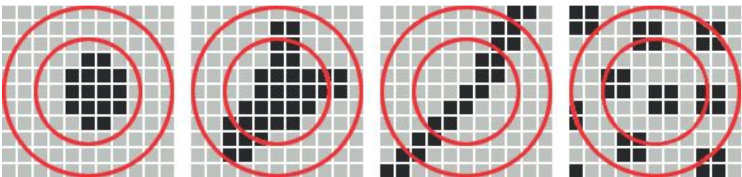
Figure 4.35 Operation of the top hat filter: Any feature contained entirely within the inner region (“crown”) is detected as in the first example. Features that are too large for the crown or are not separated by more than the width of the brim are not.
