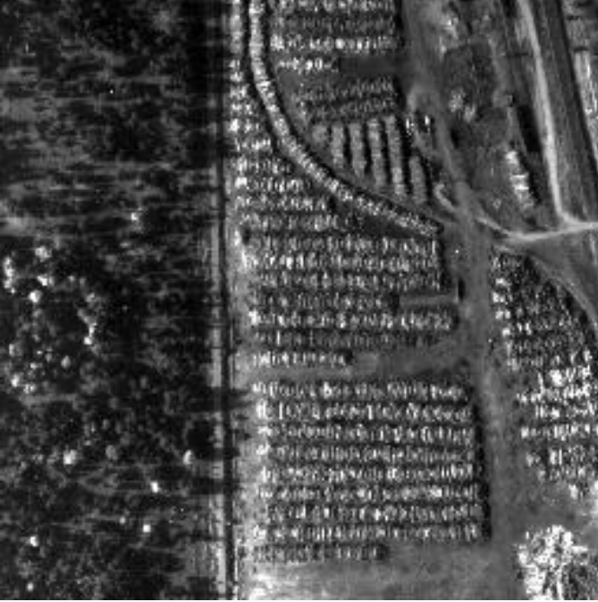
Figure 1.77 Aerial photograph in which length of shadows and knowledge of the sun position permit calculation of the heights of trees and the height of the piles of logs in the lumberyard, from which the amount of wood can be estimated.
