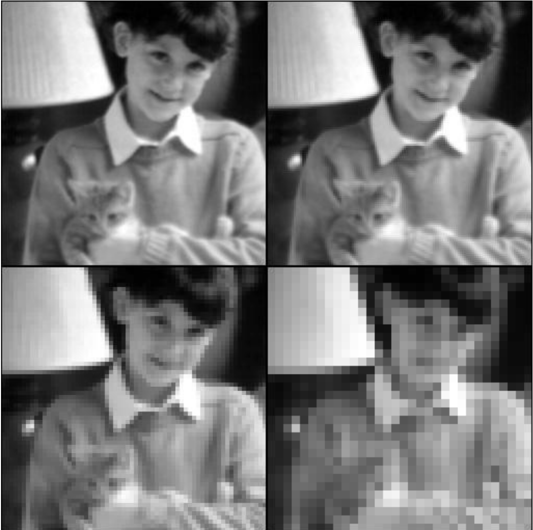
Figure 1.24 Four representations of the same image, showing a variation in the number of pixels used. From the upper left: 256 \times 256 ; 128 \times 128 ; 64 \times 64 ; 32 \times 32 . In all cases, a full 256 gray values are retained. Each step in coarsening of the image is accomplished by averaging the brightness of the region covered by the larger pixels.
