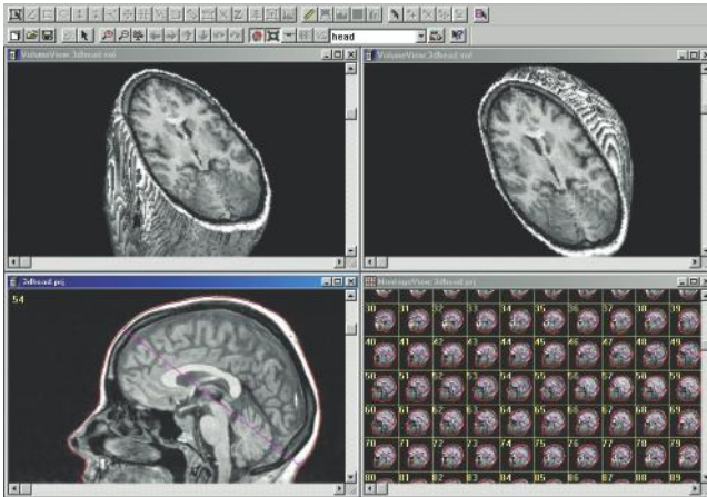
Figure 14.20 Presentation of section images, 3D reconstruction, and arbitrary plane slice on a desktop computer (courtesy of Able Software, Lexington, MA).
