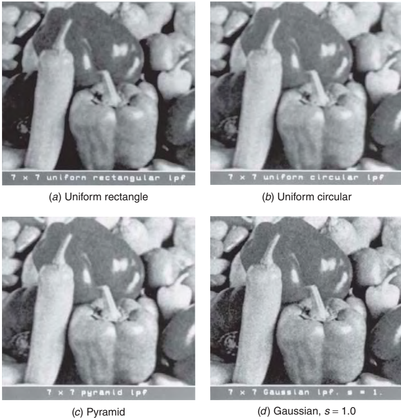
FIGURE 10.3-3. Noise cleaning with 7 \times 7 impulse response arrays on the noisy test image with uniform noise.
