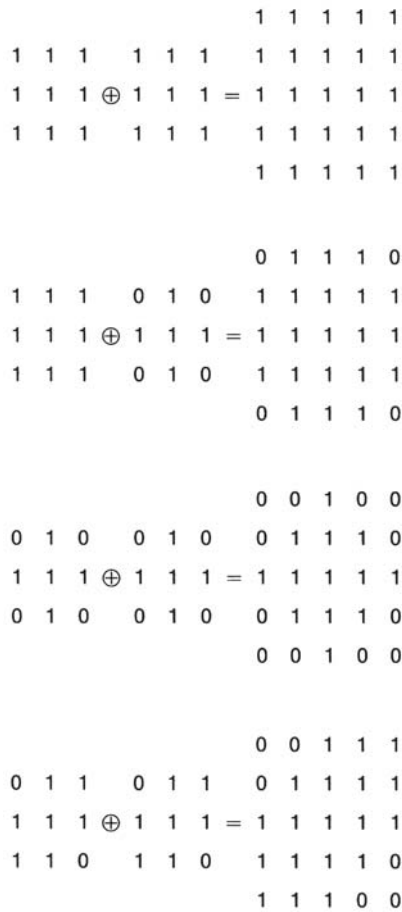
FIGURE 14.4-7. Structuring element decomposition.
