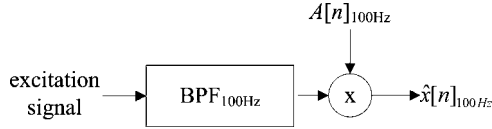
Fig. 3.19. Single channel: center frequency at 100 Hz strip of a channel vocoder (synthesis).
