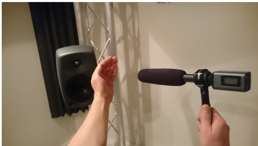
Fig. 18.4 Using a hand between speaker and microphone to obstruct the feedback path, affecting the spectral balance of the feedback signal
