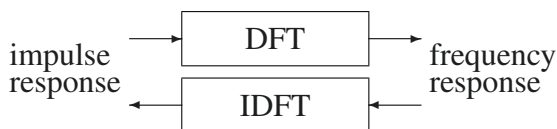
Fig. 14.5 The relationship between impulse response and frequency response of a digital filter
