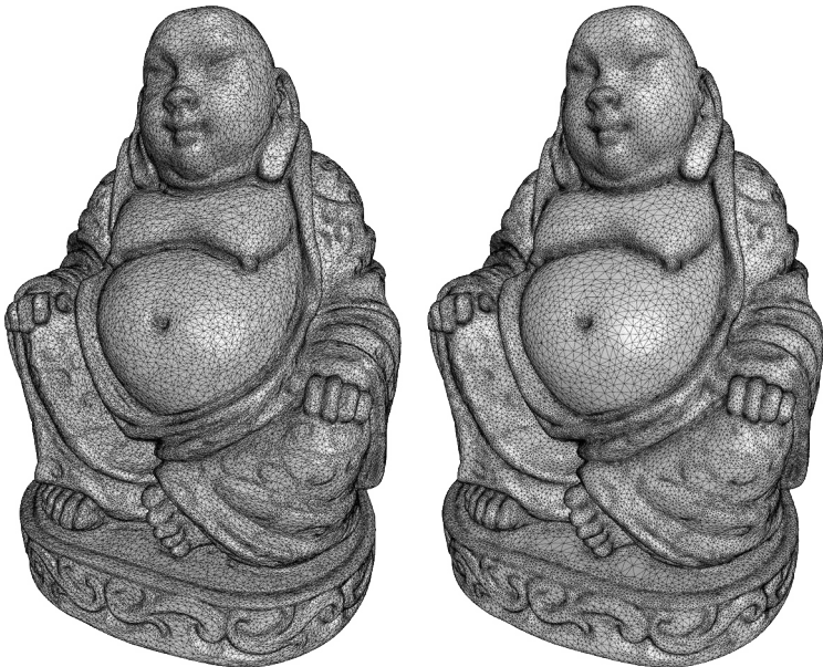
Figure 6.7. Remeshing by Delaunay refinement and filtering. The input (left) is an irregular surface triangle mesh obtained by surface reconstruction followed by simplification. The output (right) is an isotropic surface triangle mesh where all triangle angles are greater than 25 degrees. (Model courtesy of Pisa Visual Computing Lab.)
