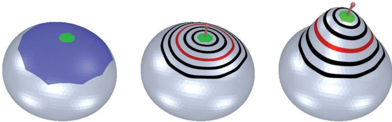
Figure 9.2. After specifying the blue support region and the green handle region (left), a smooth scalar field is constructed that is 1 at the handle and 0 outside the support (center). Its isolines are visualized in black and red, where red is the \frac{1}{2} -isoline. This scalar field is used to propagate and damp the handle's transformation within the support region (right). (Image taken from [Botsch et al. 06b]. ©2006 ACM, Inc. Included here by permission.)
