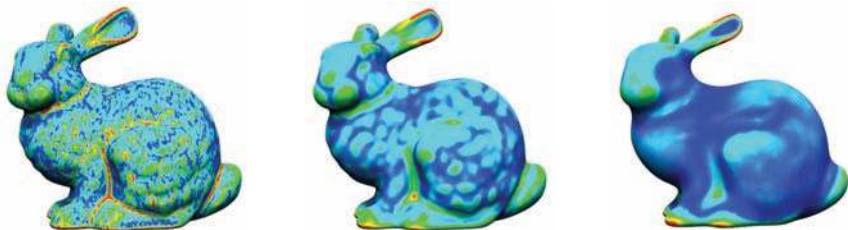
Figure 4.5. Curvature flow smoothing of the bunny mesh (left), showing the result after ten iterations (center) and 100 iterations (right). The color coding shows the mean curvature. (Model courtesy of the Stanford Computer Graphics Laboratory.)
