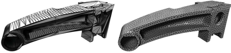
Figure 6.13. Isotropic, feature-sensitive remeshing (right) of a CAD model (left).
