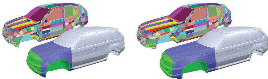
Figure 9.15. Using three independent handles allows one to stretch the car’s hood while rigidly preserving the shape of the wheel houses. This 3M triangle model consists of 10k individual connected components, which are neither 2-manifold nor consistently oriented. (Model courtesy of BMW AG. Image taken from [Botsch et al. 06b]. ©2006 ACM, Inc. Included here by permission.)
