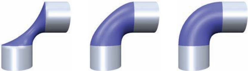
Figure 4.8. The blue region is determined by minimizing a fairness functional: membrane surface ( \Delta \mathbf{x} = 0 , left), thin-plate surface ( \Delta^2 \mathbf{x} = 0 , center), and minimum variation surface ( \Delta^3 \mathbf{x} = 0 , right). The order k of the Euler-Lagrange equation \Delta^k \mathbf{x} = 0 determines the maximum smoothness C^{k-1} at the boundary. (Image taken from [Botsch and Kobbelt 04a]. ©2004 ACM, Inc. Included here by permission.)
