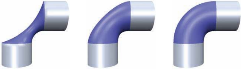
Figure 1.3. Three examples of fair surfaces, which define a blend between two cylinders: a membrane surface that minimizes the surface area (left), a thin-plate surface that minimizes total curvature (center), and a surface that minimizes the variation of mean curvature (right). (Image taken from [Botsch and Kobbelt 04a]. ©2004 ACM, Inc. Included here by permission.)
