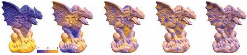
Figure 4.2. Some elements of manifold harmonic basis functions. The color values can be thought of as the amplitude of a standing wave on the mesh geometry. (Image taken from [Vallet and Lévy 08]. Model courtesy of Pisa Visual Computing Lab.)
