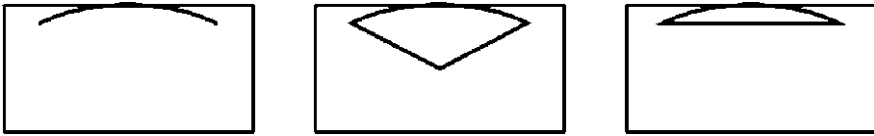
Fig. 2.12 An arc of an ellipse, a segment and an arc with its corresponding chord
