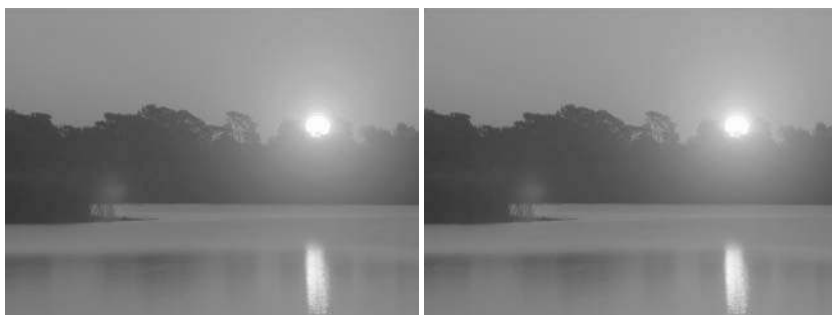
Figure 23.24. Linear interpolation for color correction. The parameter c is set to 0.0 in the left image, and to 1.0 in the right image. (See also Plate XVII.)
