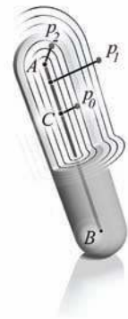
Figure 16.6. Line primitive ab and example points P_0 , P_1 , P_2 showing distance calculation.
