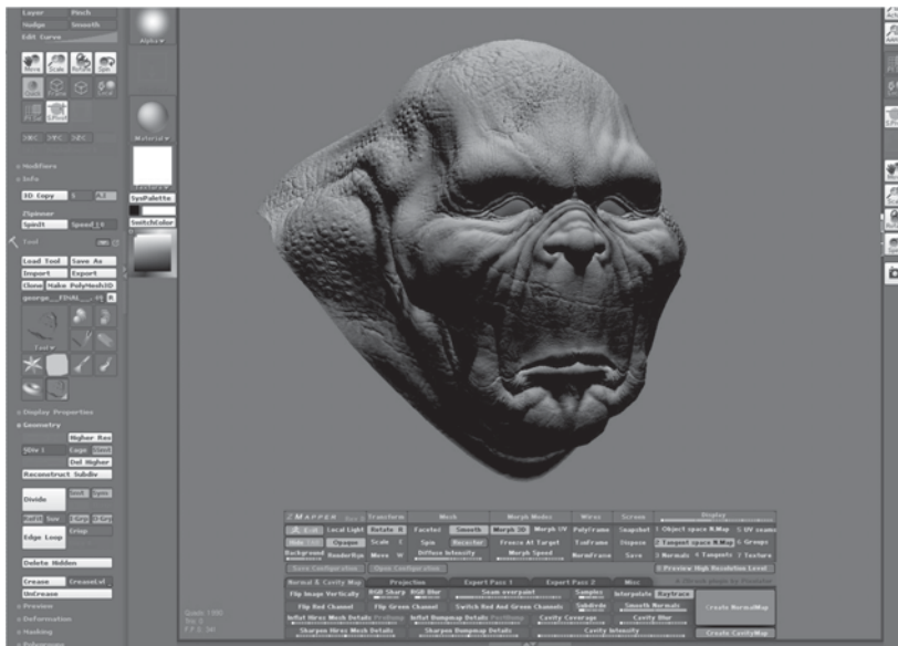
Figure 26.8. A visualization (in ZBrush) of the mesh from Figure 26.6, rendered with a normal map derived from the detailed mesh in Figure 26.7. The bottom of the figure shows the interface for ZBrush's "Zmapper" tool, which was used to derive the normal map. Image courtesy Keith Bruns.
