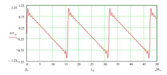
Both the ringing and the finite rise time are a result of band limiting. A perfect saw tooth would take infinite bandwidth.
