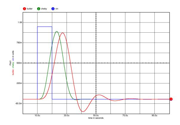
These are "real world circuits". Unlike the theoretical sinc analysis, any activity at the output can not happen before the occurrence of the input.
