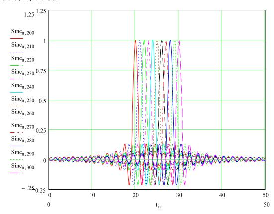
Adding the above 11 equal amplitude sinc functions yields the pulse shape below (red). Note that we are beginning to see some similarity to a band limited square wave. The blue dotted plot is a single sinc for visual reference.
