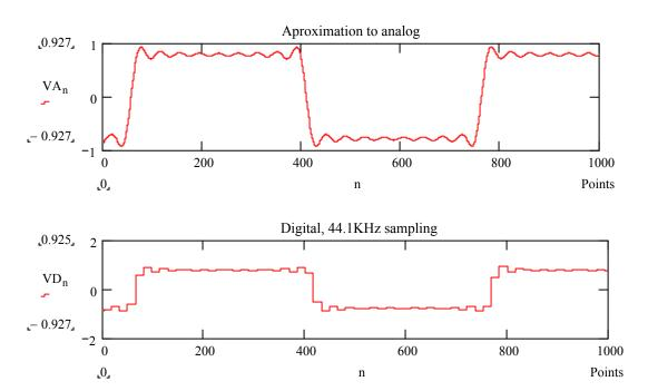
Let us filter the digitized signal. We will again approximate an analog filter with an X16 digital approximation.
