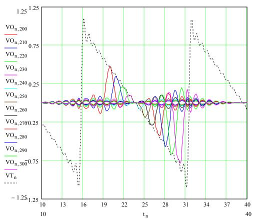
Let us complete the process by adding ALL the sincs functions. Again we see some distortions at the abrupt start (near t=0) and the end (t=50). The more abrupt, the bigger the distortion.
