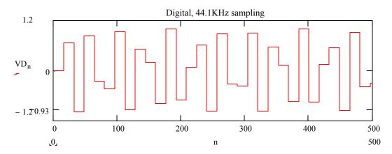
Let us filter the above digitized (sampled) signal. We will again approximate an analog output with an X16 digital approximation. Below are filter response plot (0-100KHz) and the output waveform, which again looks like a 17KHz "analog tone"
