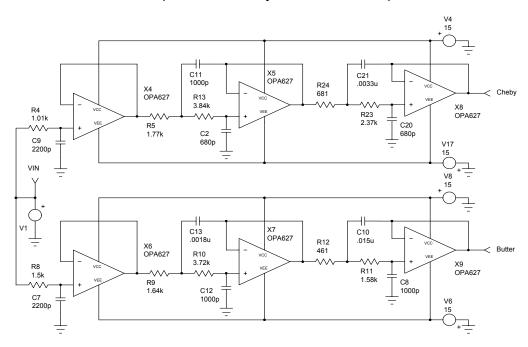
Let us make the input V1 into a sine wave and sweep over 0 to 1MHz and plot the frequency response (red - Butterworth, green – Chebyshev):
