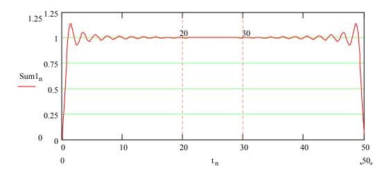
Let us find the set of sinc functions that correspond to a 3KHz sine wave. We begin by plotting the wave:
