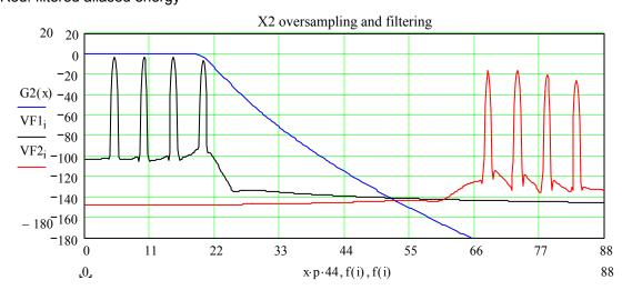
Note the additional advantage of over sampling: the attenuation of high frequency audio is reduced. The faster we over sample the less high frequency audio band attenuation. The plot below shows the improvement in flatness response for increased over sampling ratios. As mentioned before, this attenuation is due to NRZ sampling. Notice the attenuation near 20KHz:
