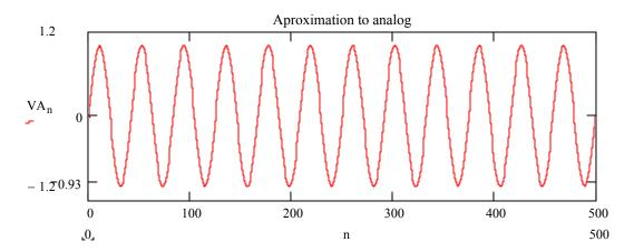
The 17KHz sine wave does not look like much of a sine wave:
