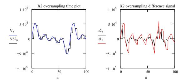
With X2 sampling, both AD alias protection requirement and DA high frequencies image removal are located at much higher frequencies thus pre and post filtering is much easier. The undesirable high frequency attenuation due to NRZ sampling has been reduced as well
