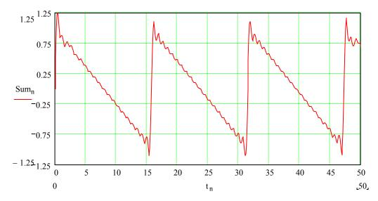
Let's find the difference between the original band limited wave and the sum of the sincs. The plot below shows the difference magnified by X10. Note that the error converges to zero at around t=25. The center point T=25 is only 25 sinc's away from the start and stop points.
