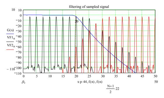
Removing high frequency BEFORE sampling (above Nyquist) is needed to avoid aliasing. We will next see that sampling itself introduces high frequency energy. The high frequency energy is "carried along" with the digital signal, but can be removed later.
