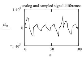
Most of the energy in the error signal is made of frequencies above the audio band, but some of that energy causes attenuation at audible high frequencies.
