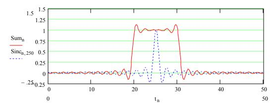
Let's add 22 adjacent sincs. 22 because this will yield a half cycle width of a 1KHz square wave. The red wave bellow shows the outcome - a positive half of a band limited square wave. The blue wave is the band limited 1KHz square wave we constructed by adding 22 sine waves. (see the first plot in this paper). Note the similarity of the positive half of the waves (ignoring the horizontal shift in time).
