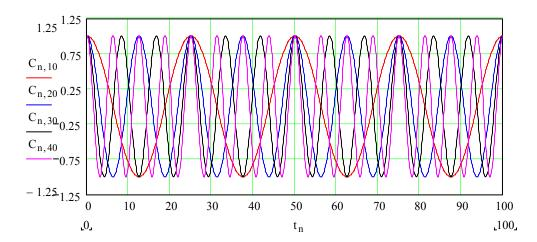
Adding the 4 waves yields and interesting result. We see the 4 waves reach their maximum value at t=0, t=25 and t=50, t=75 and t=100. This is where the added outcomes peak. Conversely, at say t=13, while two waves are peaked, the other two waves are at a minimum value, making the sum at t=13 zero. The sum of the 4 waves begins to look like a crude approximation of repeated sinc functions, such as we use for sampling:
