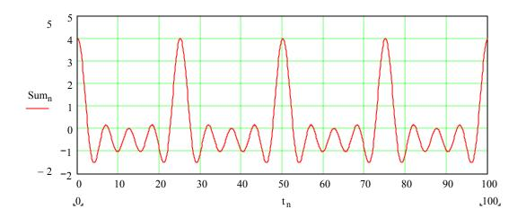
Let us double the number of cosine wave. Our Bandwidth is still 4Hz, but we now have 8 waves separated by 1/2Hz. The frequencies are 1/2Hz, 1Hz, 1.5Hz, 2Hz, 2.5Hz....4Hz. Again, we use cosine wave (phase shifted sine waves) because we want the peaks to line up and add up to a "main lobe".
