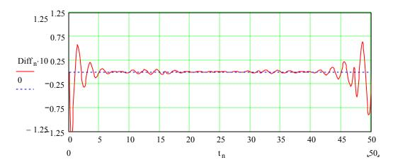
Once again, the errors near the ends (start and stop) are due to the high frequency content near the ends of the input signal. Keep in mind that the error is a high frequency signal.
