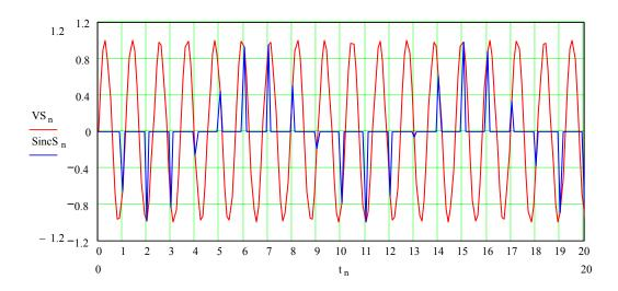
In the previous plot, the occurrence of the sinc's is too slow to track the fast changing input wave. Let's slow the input wave to less than half the sampling frequency. The sinc's location is now properly set to track the waveform.
