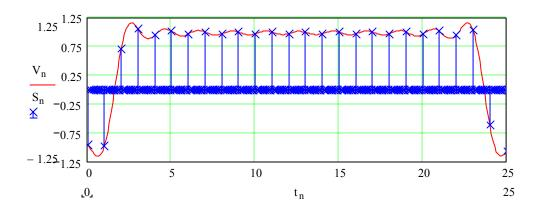
Initial intuitive reaction may cause one to think that we do not have enough X's to be able to re plot the original wave (red) with all of its details. That intuitive reaction is wrong. The key here is fact that the wave form is band limited. For a given bandwidth, the number of samples (X's) need only to exceed twice the bandwidth in order to be able to retrieve the complete waveform, including any value between the sample times. Let us see how it is done.
