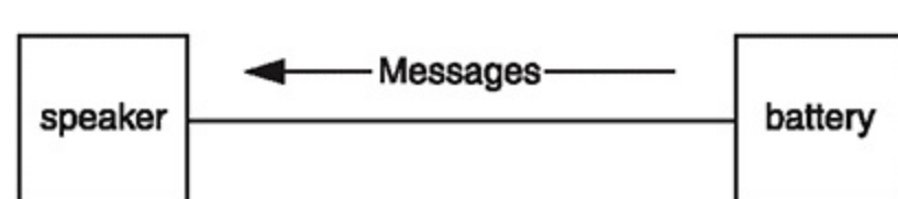
Figure 1.1. This simple telegraph network transmits electrical signals from one end to the other.
