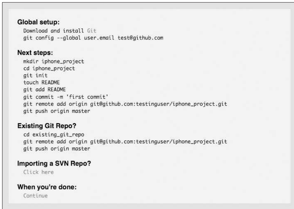
Figure 4-7. Instructions for a new repository
