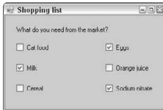
Figure 10-10: Check boxes can display multiple choices and pick more than one option.
