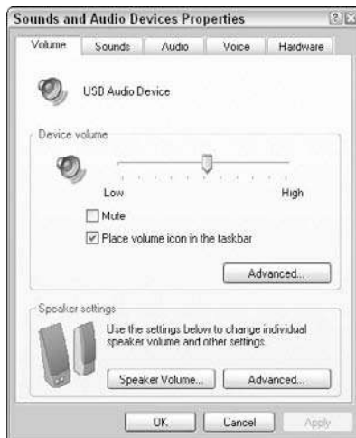
Figure 10-13: A slider lets users visually choose a numeric value or setting by dragging a slider along a ruler.
