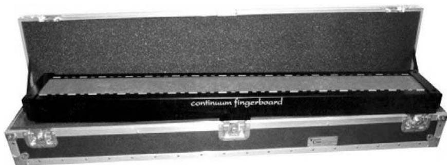
FIGURE 3.7. The Continuum Fingerboard is approximately the same size as a traditional music keyboard, but it has no discrete keys. It has a pitch range of nearly eight octaves. The white markings indicate the white key pattern of a traditional keyboard.
