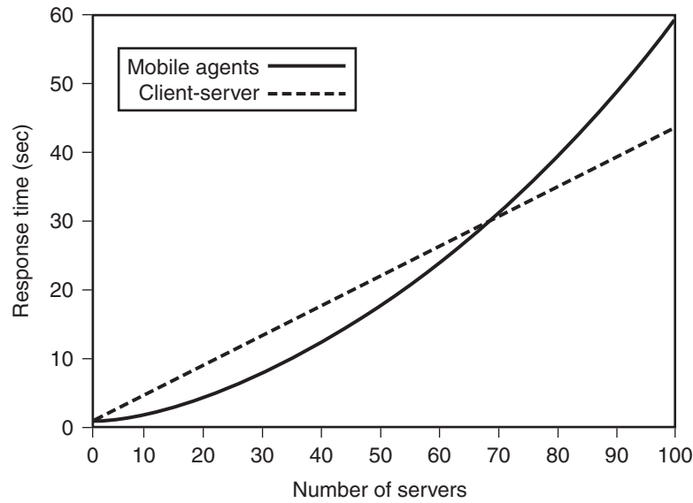
Figure 3.8 Evaluation of Scenario 3.4: Response time versus number of servers. The number of servers for which response time of client-server and mobile agents are equal is higher than in Scenario 3.3.
