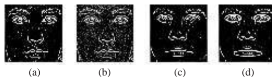
Figure 1. Edge detection, (a) 15x15 LOG, (b) 7x7 LOG, (c) 7x7 LOG and median filter, (d) best fitting ovals around the eyes and mouth
