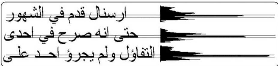
Figure 1.8 Horizontal projection profile for a given Arabic text.
