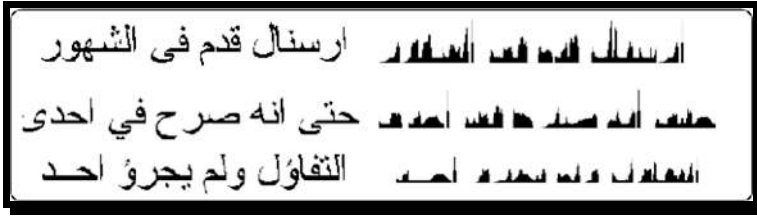
Figure 1.9 Vertical projection profile for a given Arabic text.
