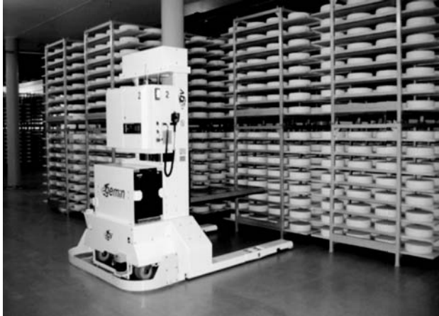
FIGURE 6.4 An AGV in a cheese factory.
