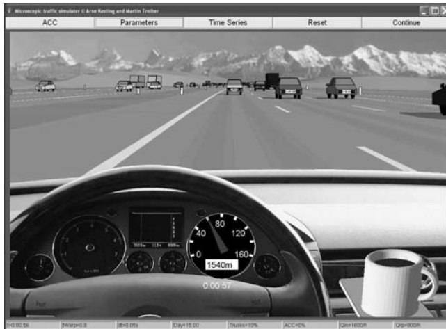
FIGURE 11.11 Example of a 3D animation from the driver perspective. Notice that the “Coffeemeter” visualizes the acceleration and the jerk (the changes of all acceleration with time) which are difficult to visualize by other means. It therefore serves as a measure of the driving comfort.
