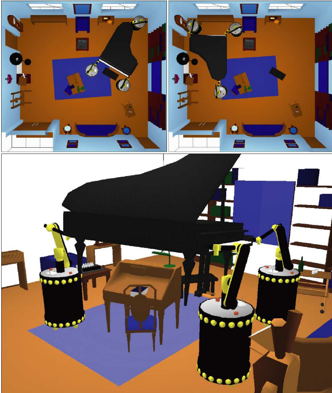
Figure 1.3: Using robots to move a piano [177]. This solution was computed using planning techniques developed by Juan Cortés, Thierry Simeon, and Jean-Paul Laumond, and are covered in Section 7.4.
