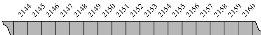
Figure 5.1: A representation of a portion of a computer’s memory, with individual bytes labeled with consecutive memory addresses.
