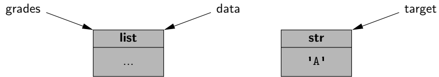
Figure 1.7: A portrayal of parameter passing in Python, for the function call count(grades, 'A') . Identifiers data and target are formal parameters defined within the local scope of the count function.
