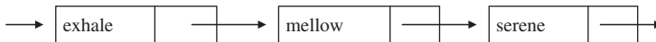
FIGURE 4.2 Part of a linked collection—a singly-linked list —in which each entry contains an element and a reference to the next entry in the linked collection
