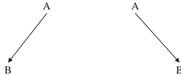
FIGURE 15.7 Two distinct binary trees, one with an empty right subtree and one with an empty left subtree
