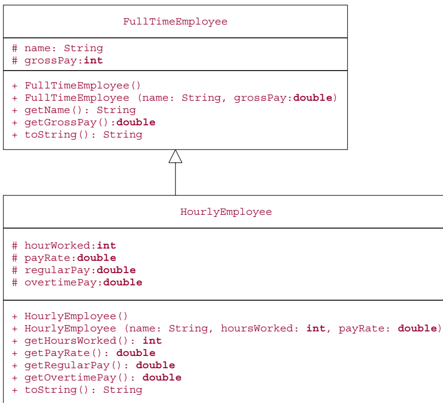
FIGURE 1.2 In UML, the notation for inheritance is a solid arrow from the subclass to the superclass
