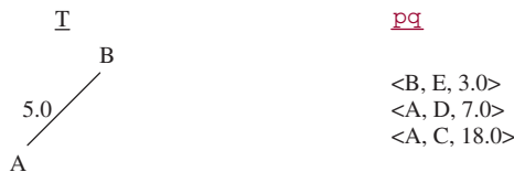
FIGURE 15.18 The contents of T and pq during the application of Prim's algorithm to the network in Figure 15.14
