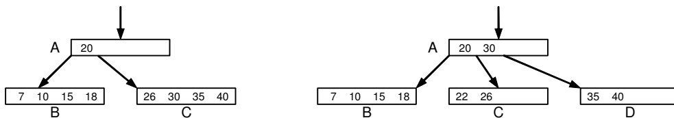
Fig. 4.44. Insertion of key 22 in B-tree
